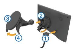
2 Press the mount ② onto the suction cup ③ until it snaps into place.
